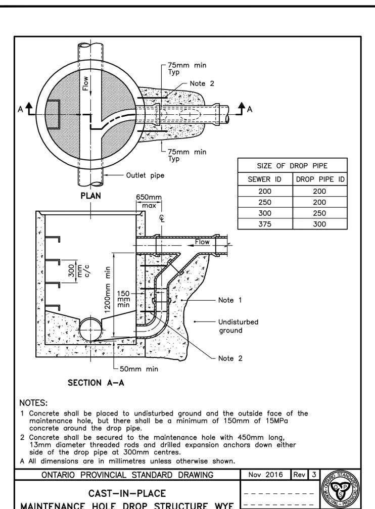
CAST-IN-PLACE MAINTENANCE HOLE DROP STRUCTURE WYE
