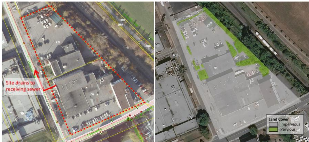
Figure 2: Existing Drainage (left) and Land Cover (right)
