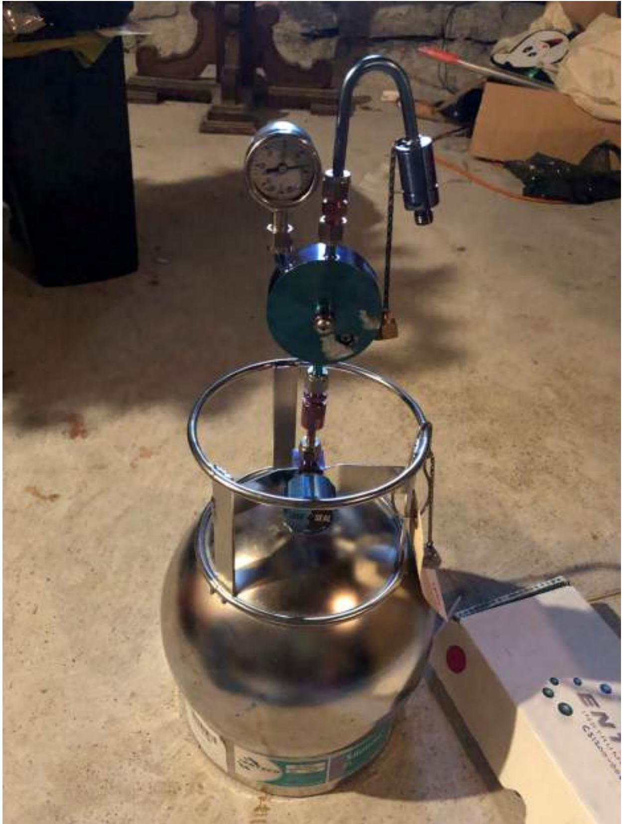
*Image 8 – Air canister sampling at 250 Rochester Street (Indoor250)*
