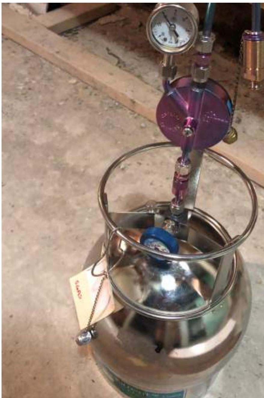
*Image 1 – Air Canister Sampling at 254 Rochester Street (Indoor254)*
