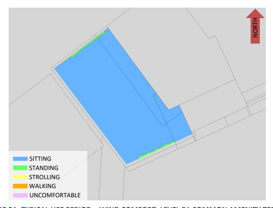
FIGURE 8A: TYPICAL USE PERIOD – WIND COMFORT, LEVEL B1 COMMON AMENITY TERRACE
