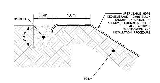
ANCHORING DETAIL FOR POND LINER NTS
