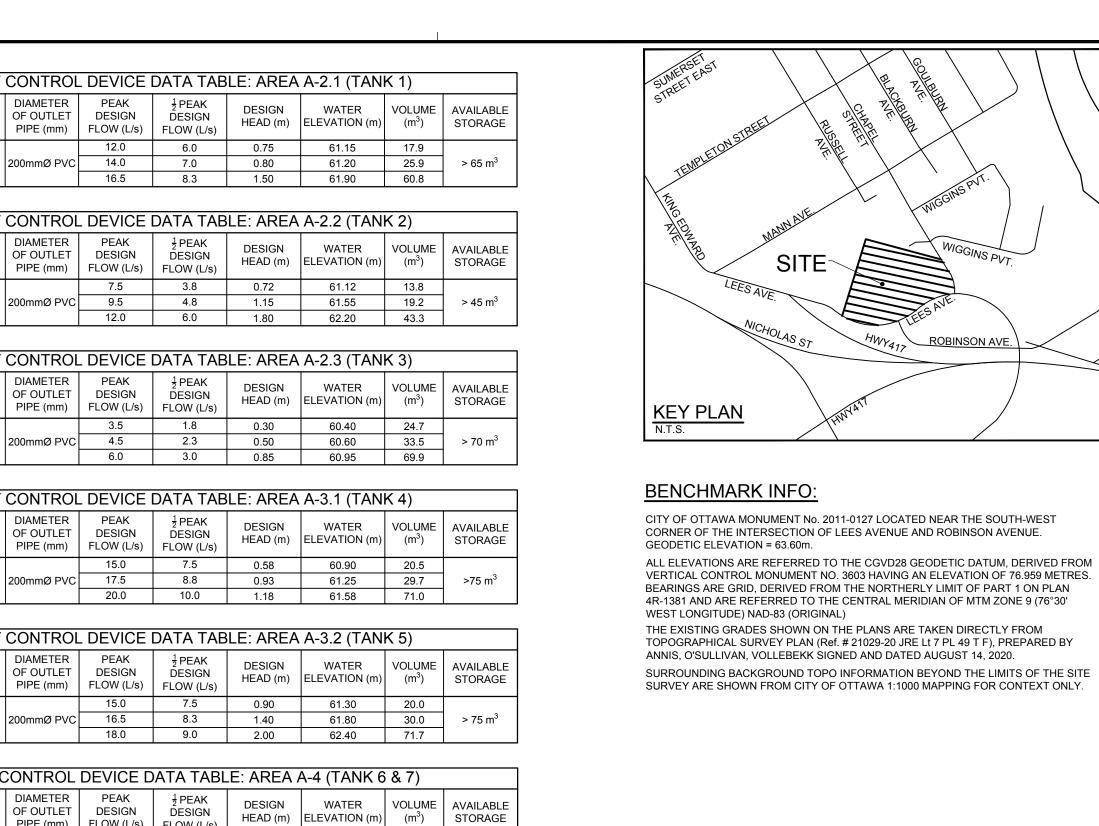
INLET CONTROL DEVICE DATA TABLE: AREA A-2.1 (TANK 1)
