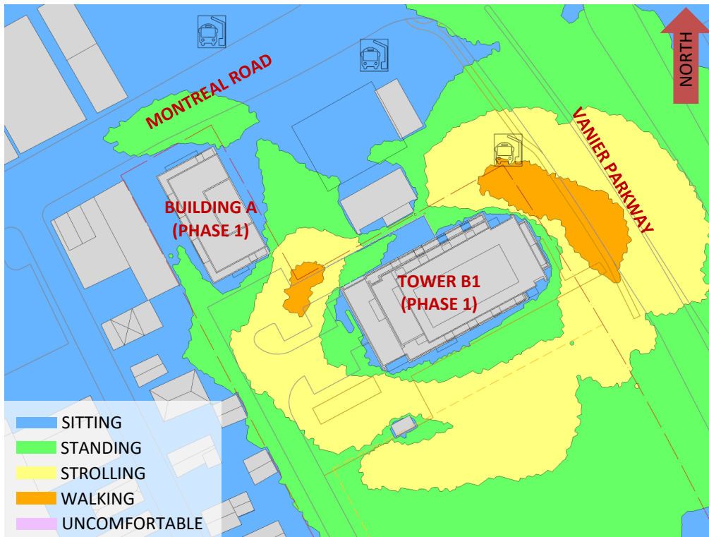
FIGURE 3B: SPRING – PHASE 1 – WIND COMFORT, GRADE LEVEL
