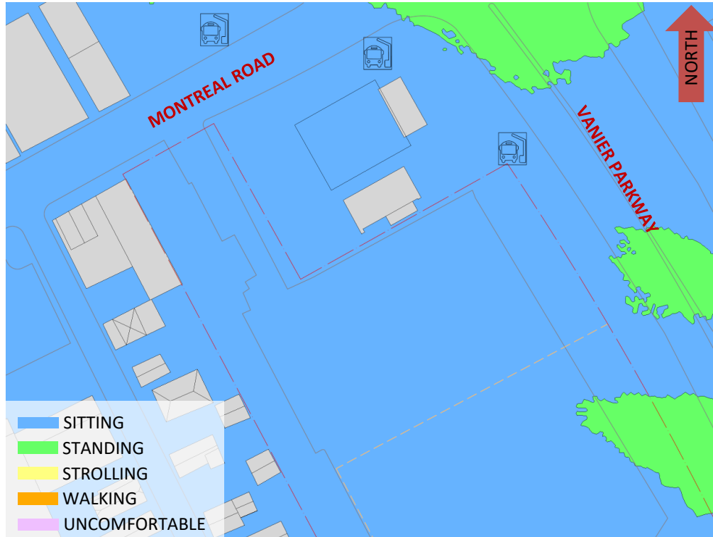
FIGURE 3C: SPRING – EXISTING MASSING – WIND COMFORT, GRADE LEVEL
