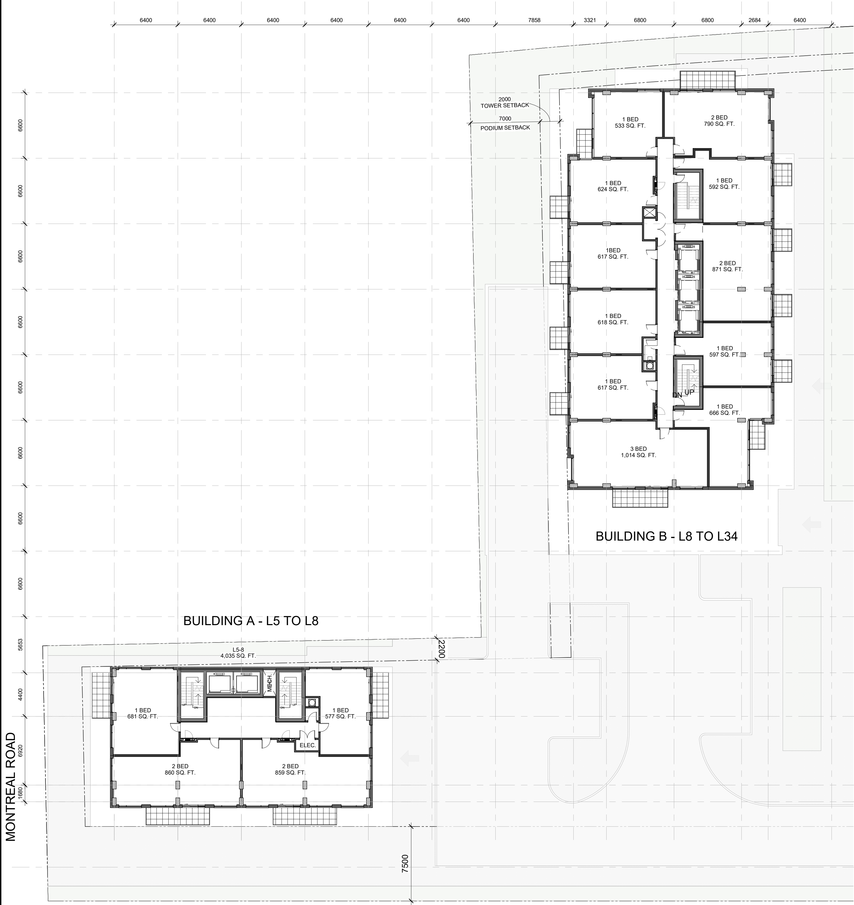
1 BUILDING A - 5TH TO 8TH AND BUILDING B - 8TH TO 34TH FLOOR PLAN 1 : 200
