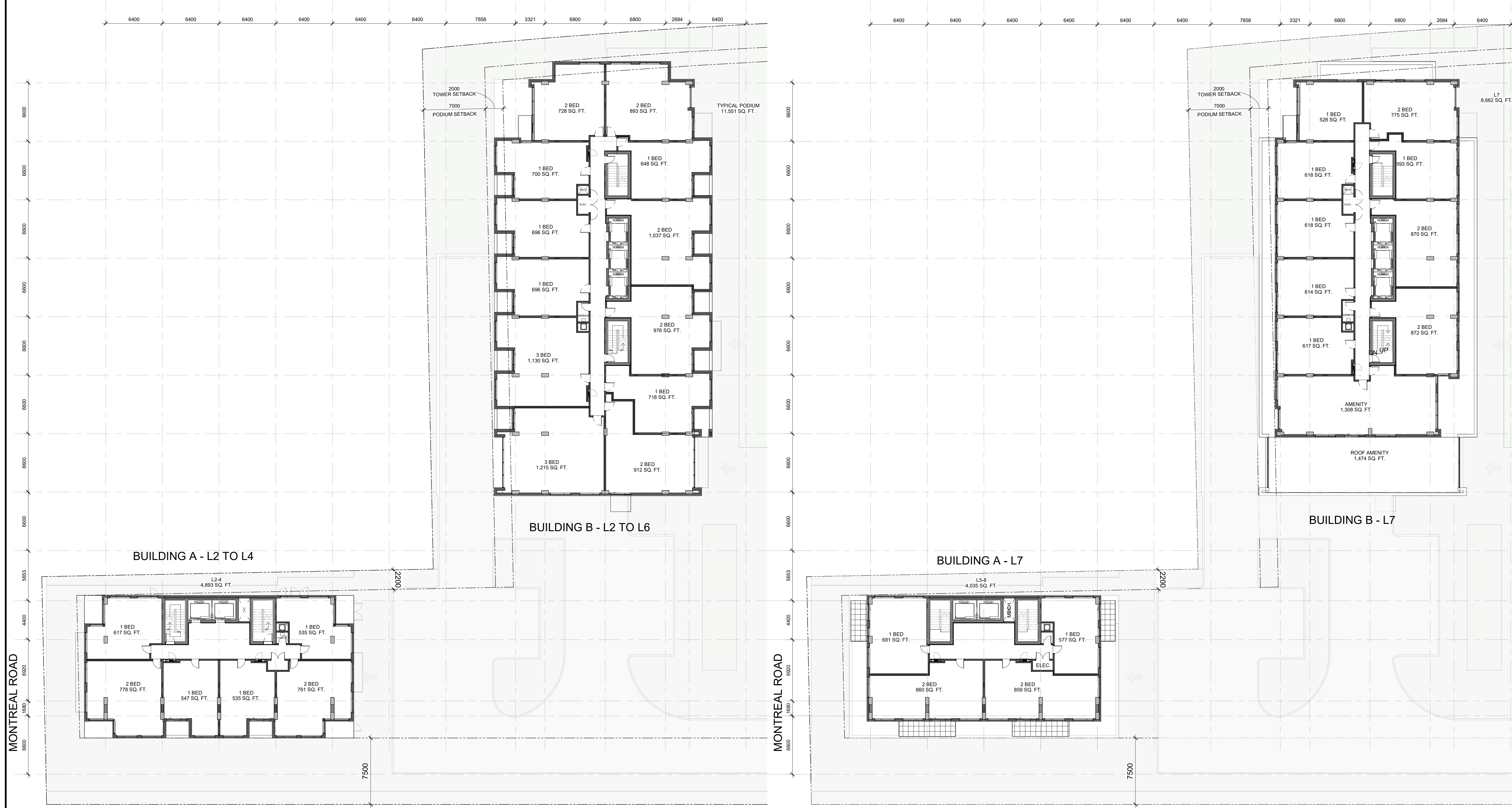
1 BUILDING A - 2ND TO 4TH AND BUILDING B - 2ND TO 6TH FLOOR PLAN 1 : 200
