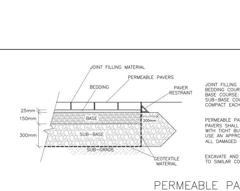
JOINT FILLING MATERIAL: 2.5-10mm AGGREGATE OR AS RECOMMENDED BY MANUFACTURER BEDDING COURSE: 2.5-10mm AGGREGATE OR AS RECOMMENDED BY MANUFACTURER BASE COURSE: 5-28mm AGGREGATE OR AS RECOMMENDED BY MANUFACTURER SUB-BASE COURSE: 40-80mm AGGREGATE OR AS RECOMMENDED BY MANUFACTURER COMPACT EACH LAYER AS RECOMMENDED BY MANUFACTURER
