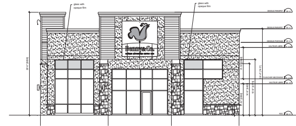
2 NORTH ELEVATION - RESTAURANT SCALE: 1:100
