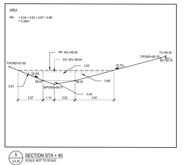
= (9.28+0)/2 = 4.64 x 2.37 = (12.23+9.28)/2 = 10.755 x 10 = (12.23+9.39)/2 = 10.81 x 10  $= 107.55 m^3$  $= 108.10 \text{m}^3$ = (9.39+7.4)/2 = 8.40 x 10  $= 84.00 \text{m}^3$ = (7.4+3.39)/2 = 5.40 x 10  $= 54.00 \text{m}^3$ = (3.39+0)/2= 1.695 x 1.29  $= 2.187 \text{m}^3$ PR. VOLUME = 366.84m<sup>3</sup>
