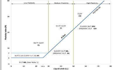
Note 1 – Fine grained materials with PI and LL that plot in this area are named (ML) SILT with slight plasticity. Fine-grained materials which are non-plastic (i.e. a PL cannot be measured) are named SILT
