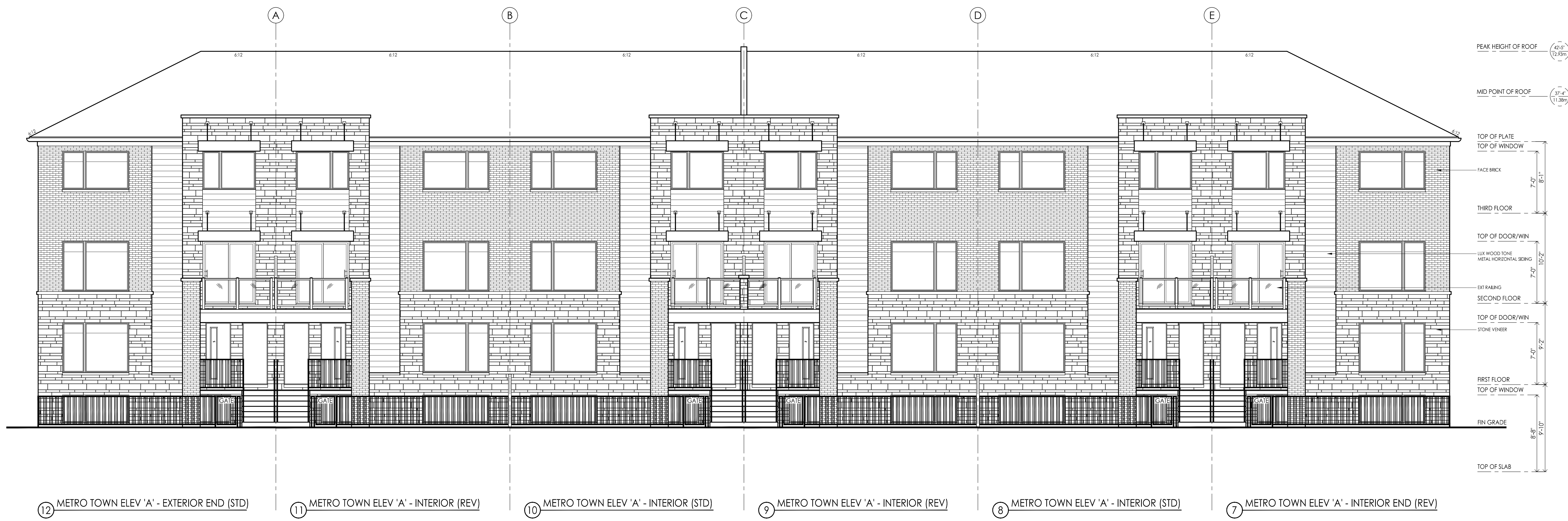
INTERIOR FRONTAGE - TYPICAL BLOCK ELEV 'A'
