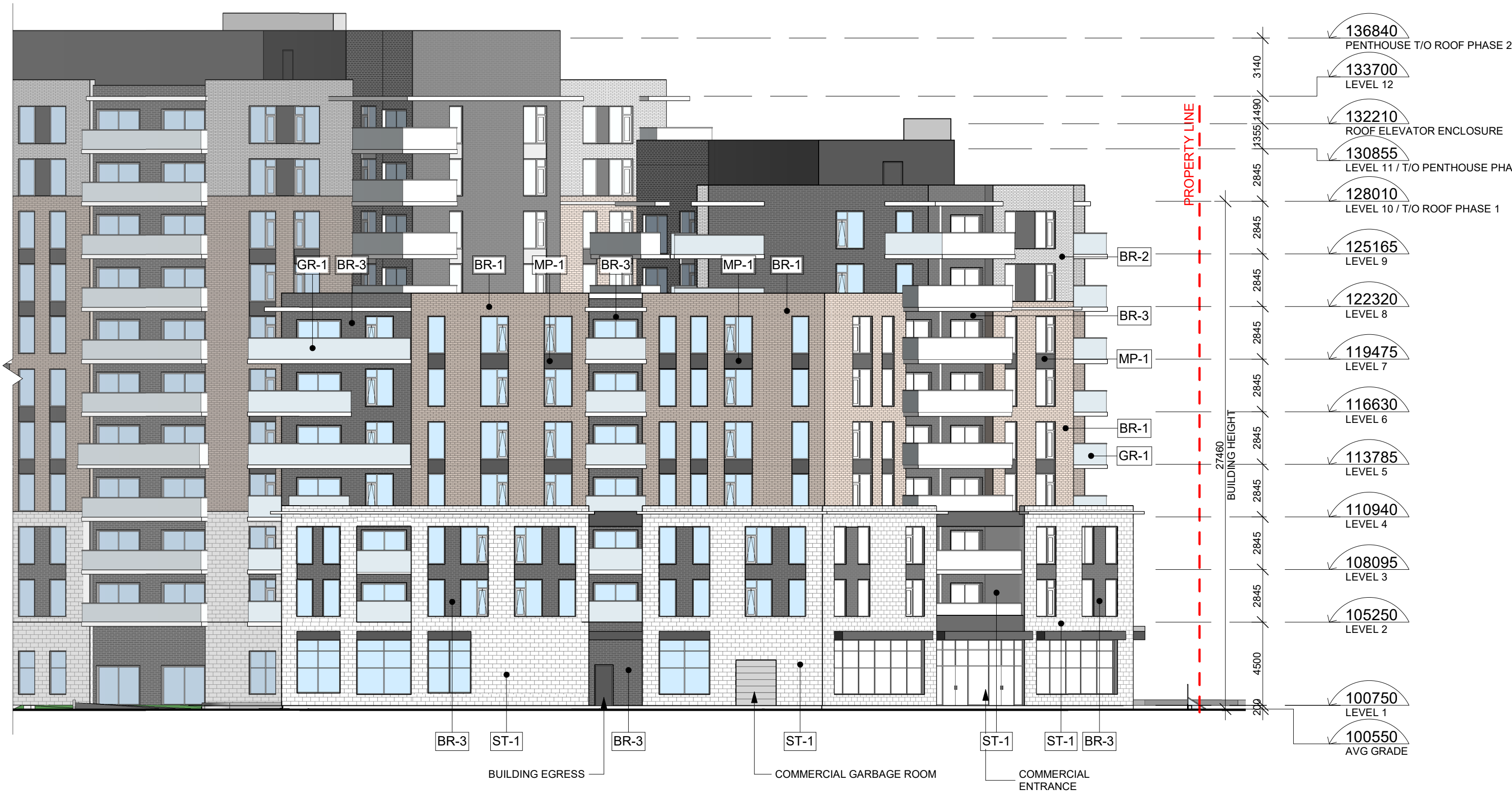
3 EAST ELEVATION - WEST WING 1 : 200
