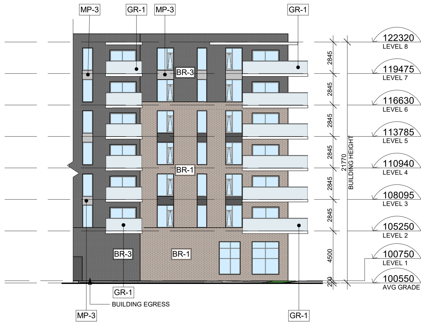
3 WEST ELEVATION - WEST BUILDING 1 : 200
