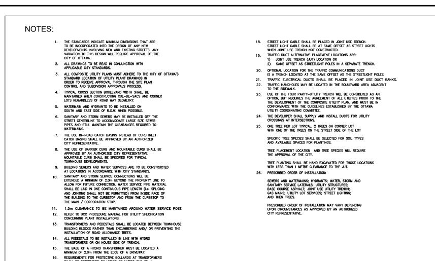
17. SERVICE LATERALS MUST BE LOCATED A MINIMUM OF 3.0m FROMTHE BASE OF A HYDRO TRANSFORMER.
