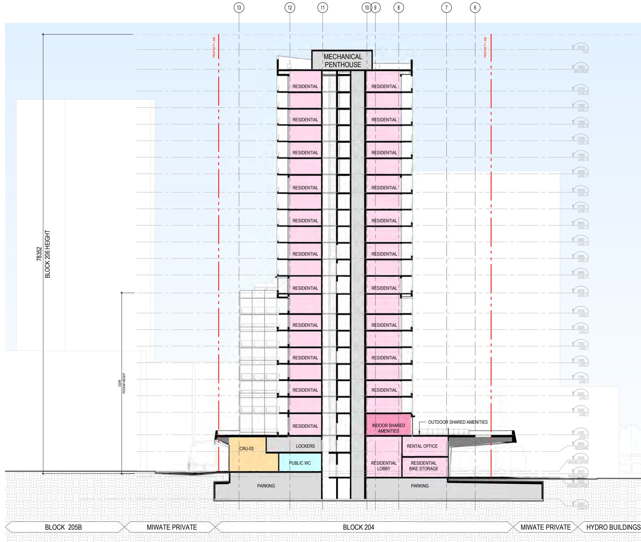
NORTH-SOUTH BUILDING SECTION
