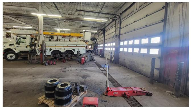
Photo 5: Facing south, moderate levels of oil stains observed on the concrete floor, floor drains leading to an Oil Water Separator present along the western portion of the building.
