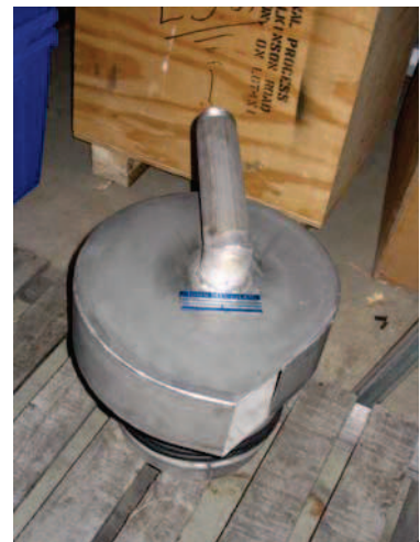
VHV with air vent for minimal slopes
