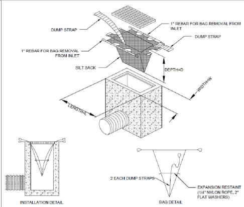
INLET SEDIMENT CONTROL DEVICE
