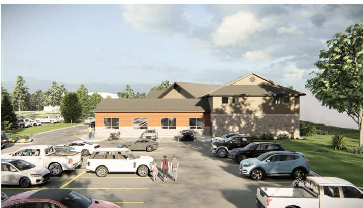
ABOVE LEFT: The majority of parking is located at the rear of the site. The parking area has been designed to ensure there are no entrapment areas. Large windows provide for natural surveillance onto this area in accordance with Crime Prevention through Environmental Design (CPTED) principles).
