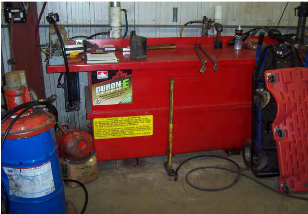
Photograph 8: Bulk new oil storage tank located in the maintenance garage.
