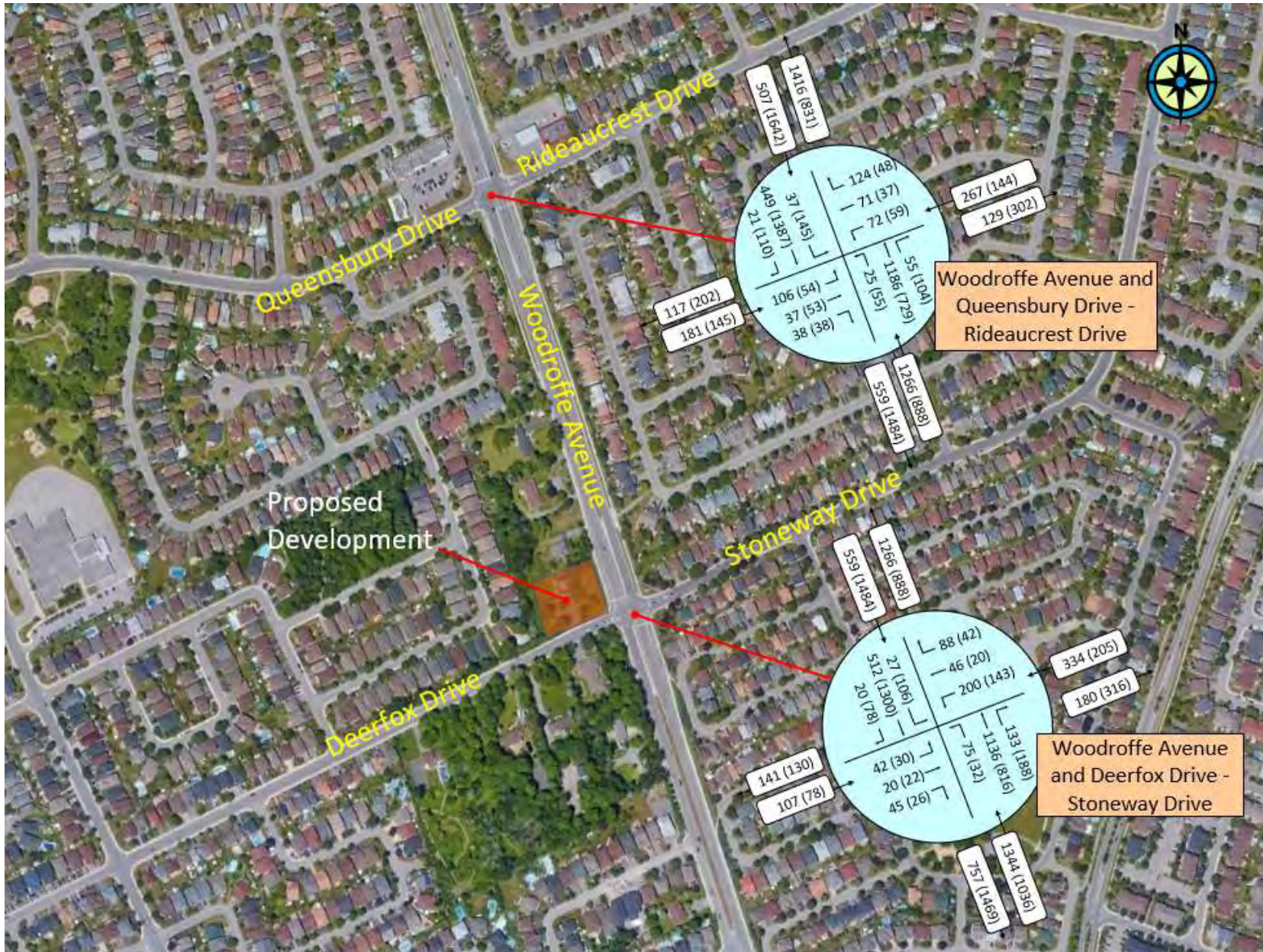
Morning (Afternoon), vph = vehicles-per-hour Exhibit 2-8: Existing (2022) Balanced Morning and Afternoon Peak Hour Traffic Volumes
