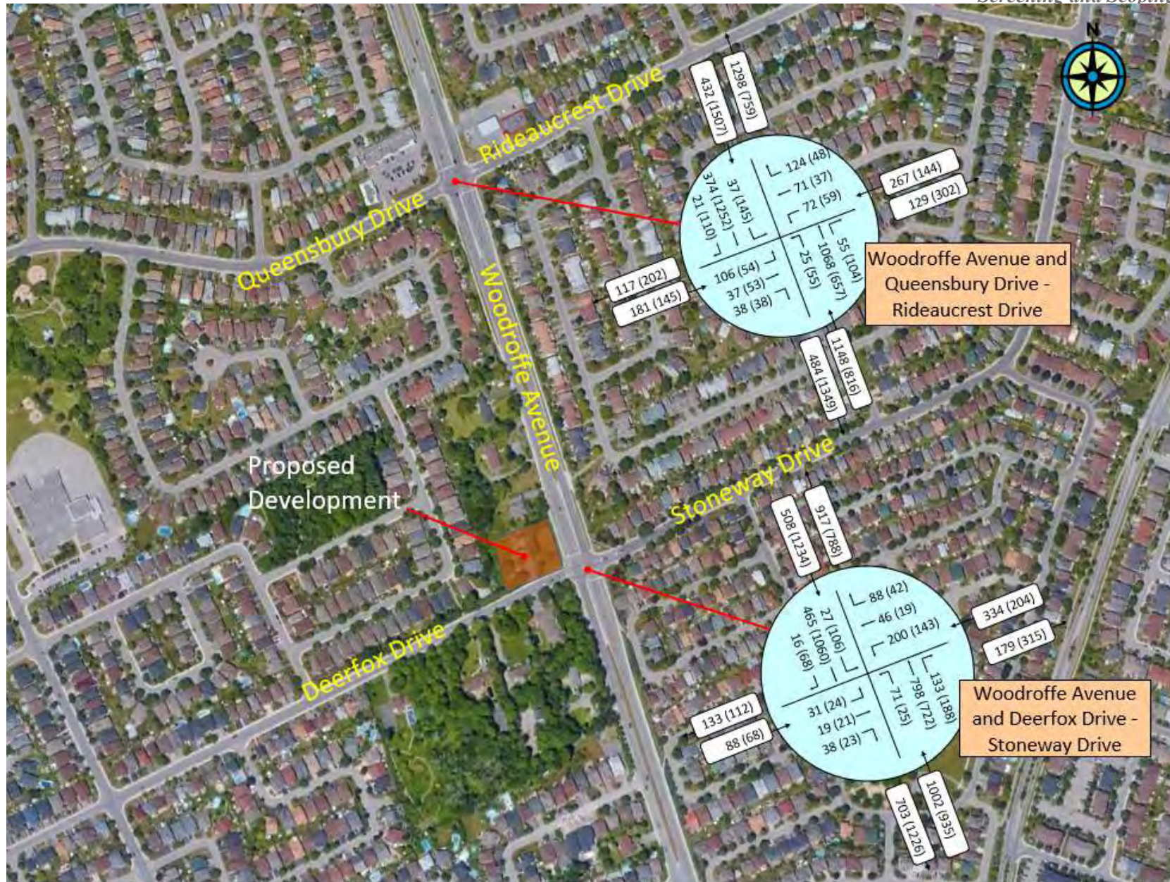
Morning (Afternoon), vph = vehicles-per-hour Exhibit 2-7: 2017 Non-Balanced Morning and Afternoon Peak Hour Traffic Volumes
