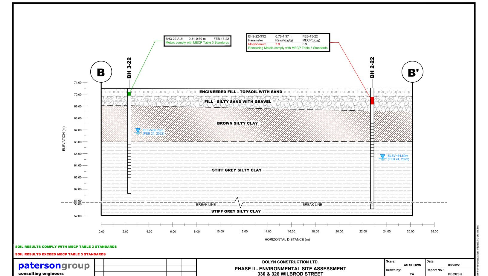
**CROSS SECTION B-B' - SOIL (METALS)**
