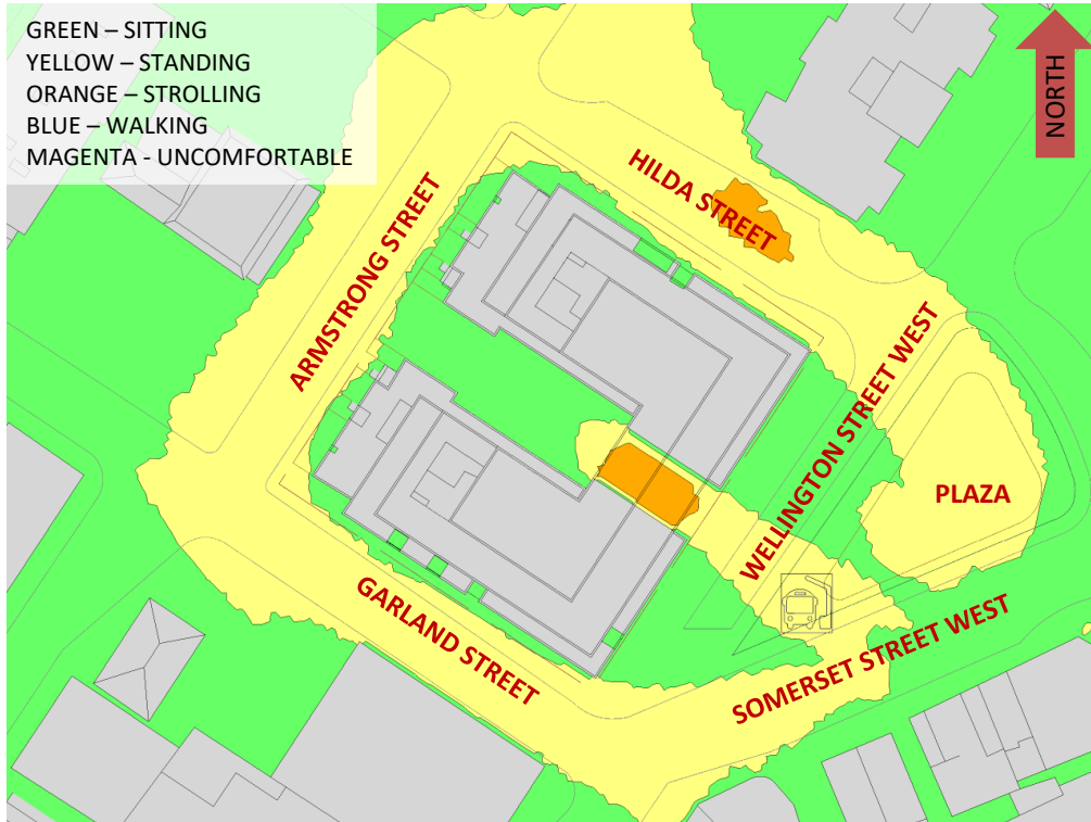
FIGURE 3A: SPRING – WIND CONDITIONS AT GRADE LEVEL
