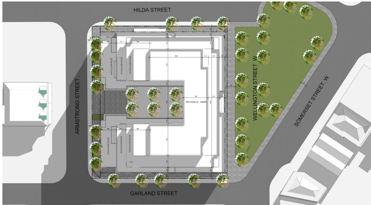
Figure 27: Ground floor plan showing the landscape treatment with retail identified in pink and residential in green. Wrapping the retail around the corner onto Garland Street along with the varied setback of the retail reinterpret the original street ambience. Source: Roderick Lahey Architect 2021.
