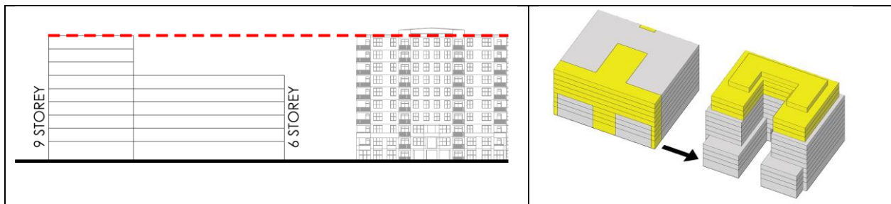
Figure 29: Zoning height relative to existing conditions and a model illustrating transfer of density has resulted in a slightly taller building from 9-storeys to 13-storeys creating a more pedestrian friendly environment. Source: rla Architect 2021.
