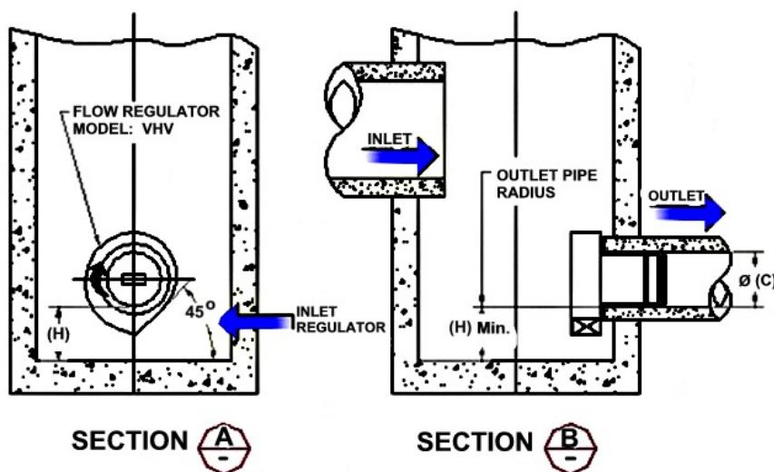
**FLOW REGULATOR TYPICAL INSTALLATION IN SQUARE MANHOLE**
