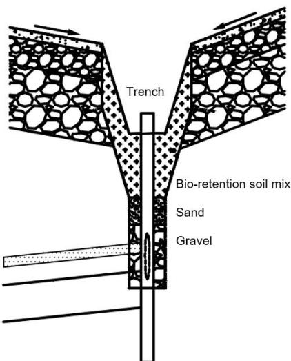
**Figure 2: Bioswale cross-section**
