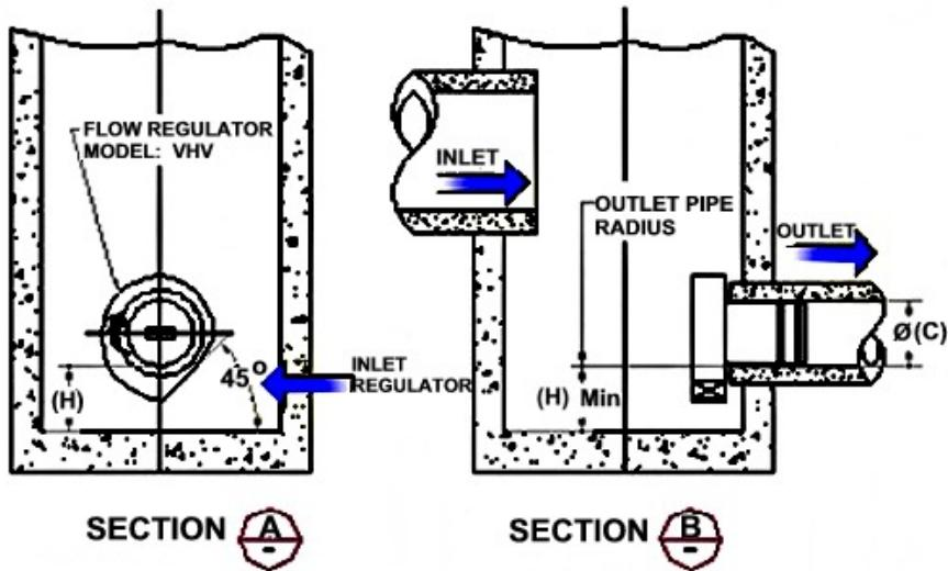
**FLOW REGULATOR TYPICAL INSTALLATION IN CIRCULAR MANHOLE**
