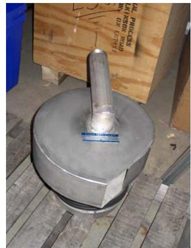
**VHV with air vent for minimal slopes**
