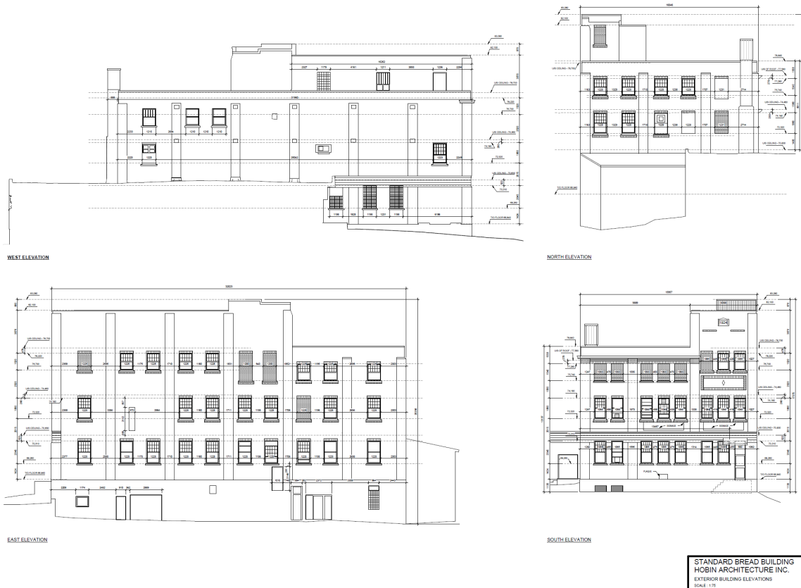
Figure 28: Dimensioned As-found record of elevation and floor plans of the Standard Bread Building. Source Hobin Architecture Inc.
