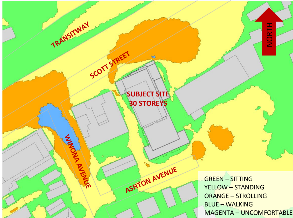
FIGURE 3A: SPRING – WIND CONDITIONS AT GRADE LEVEL
