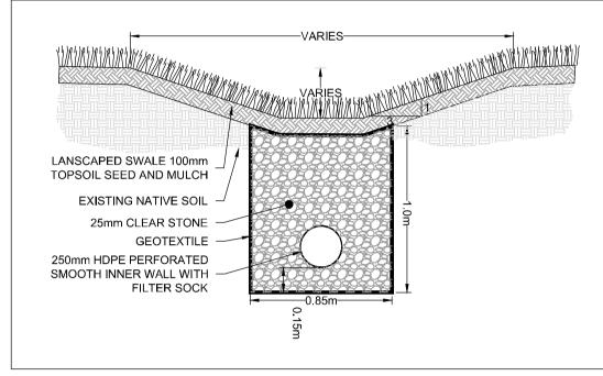
TYPICAL SWALE CROSS-SECTION DETAIL
