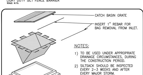
ROADSIDE CATCH BASIN PROTECTION DETAIL: TERRAFIX SILTSACK SCALE: N.T.S.
