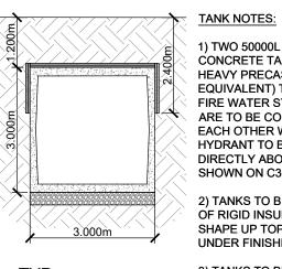
1) TWO 50000L PRECAST CONCRETE TANKS BY WILKINSON HEAVY PRECAST LTD. (OR EQUIVALENT) TO BE USED FOR FIRE WATER STORAGE. TANKS ARE TO BE CONNECTED WITH EACH OTHER WITH 200mm PIPE. HYDRANT TO BE INSTALLED DIRECTLY ABOVE TANK AS SHOWN ON C300.
