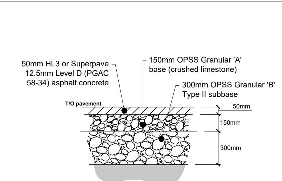
1 C3 Pavement Structure for Light Duty Traffic (Typ.)
