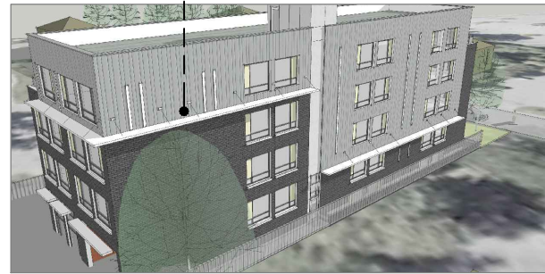
SUSPENDED OVERHANG - to define separation of materials and reduce visual scale of facade
