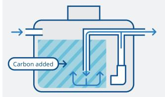
A pump re-circulates the water through the filtration media. External carbon is added
