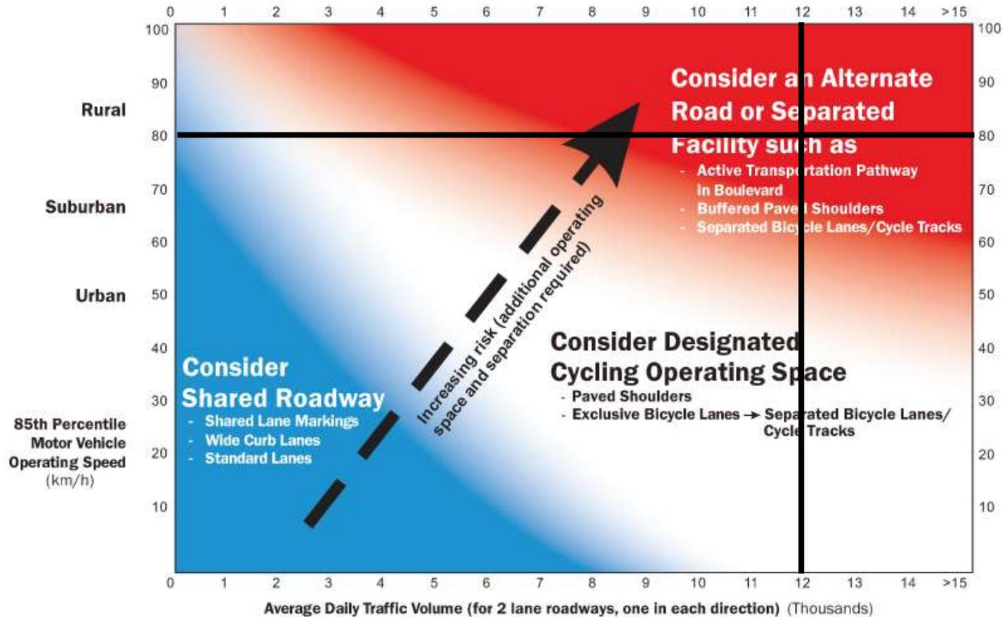
Figure 3.3 – Desirable Bicycle Facility Pre-Selection Nomograph
