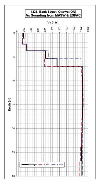
Figure 5: MASW Shear-Wave Velocity Soundings
