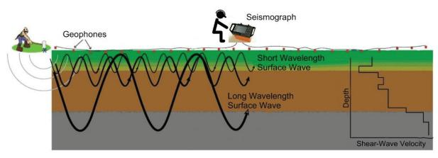
Figure 3: MASW Operating Principle
