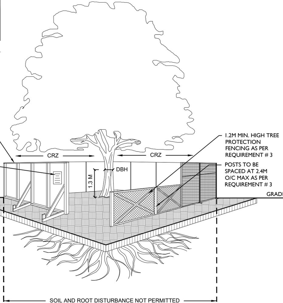
1.2M MIN. HIGH TREE PROTECTION FENCING AS PER REQUIREMENT # 3
