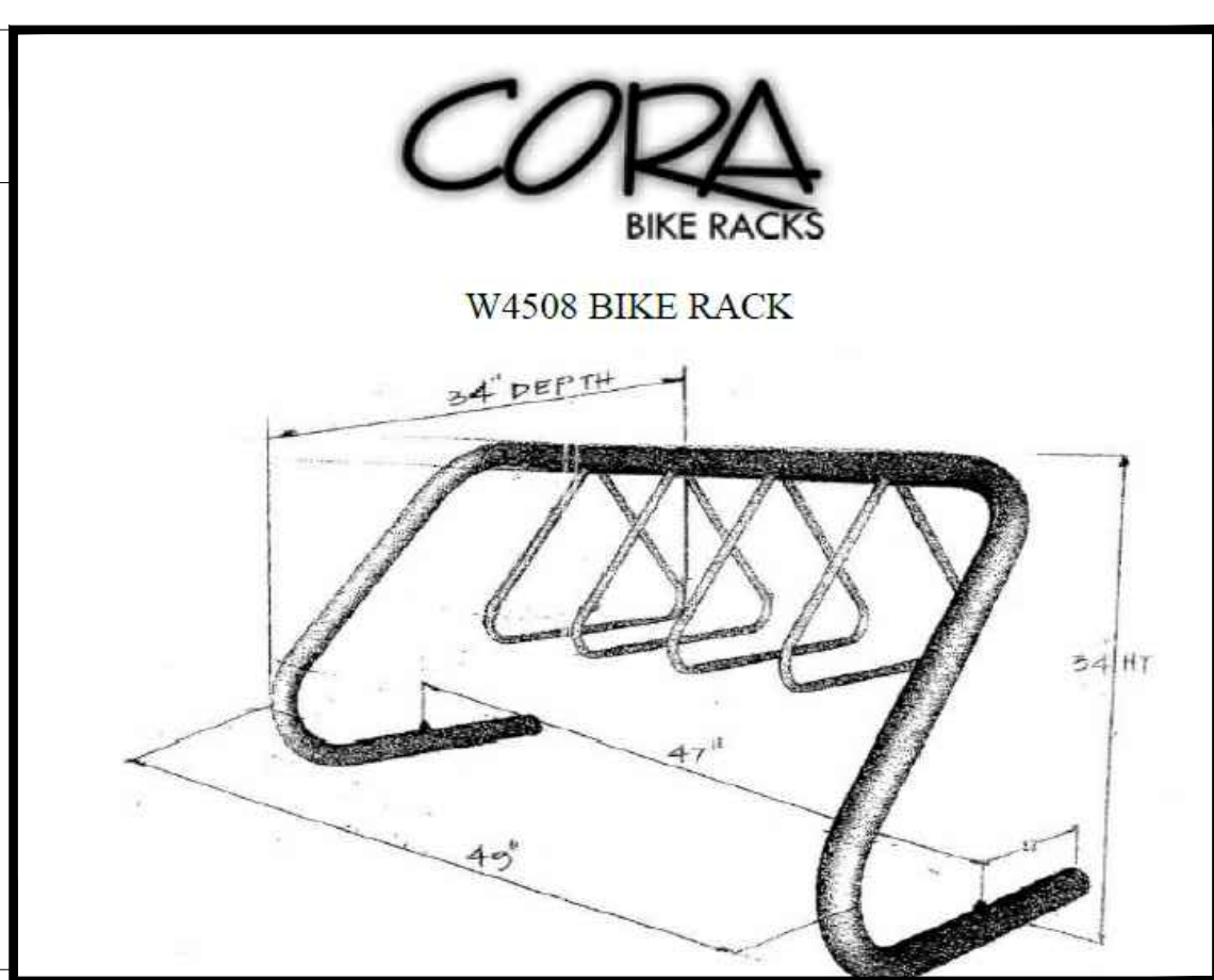
5 BIKE RACK CUT SHEET L100 / NTS
