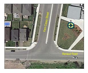
**Renaud Road/Fern Casey Street:** This "T" intersection is currently STOP-controlled on the north leg. An EB-LT auxiliary lane is provided from Renaud Road with single-lane thru movements on each approach.
