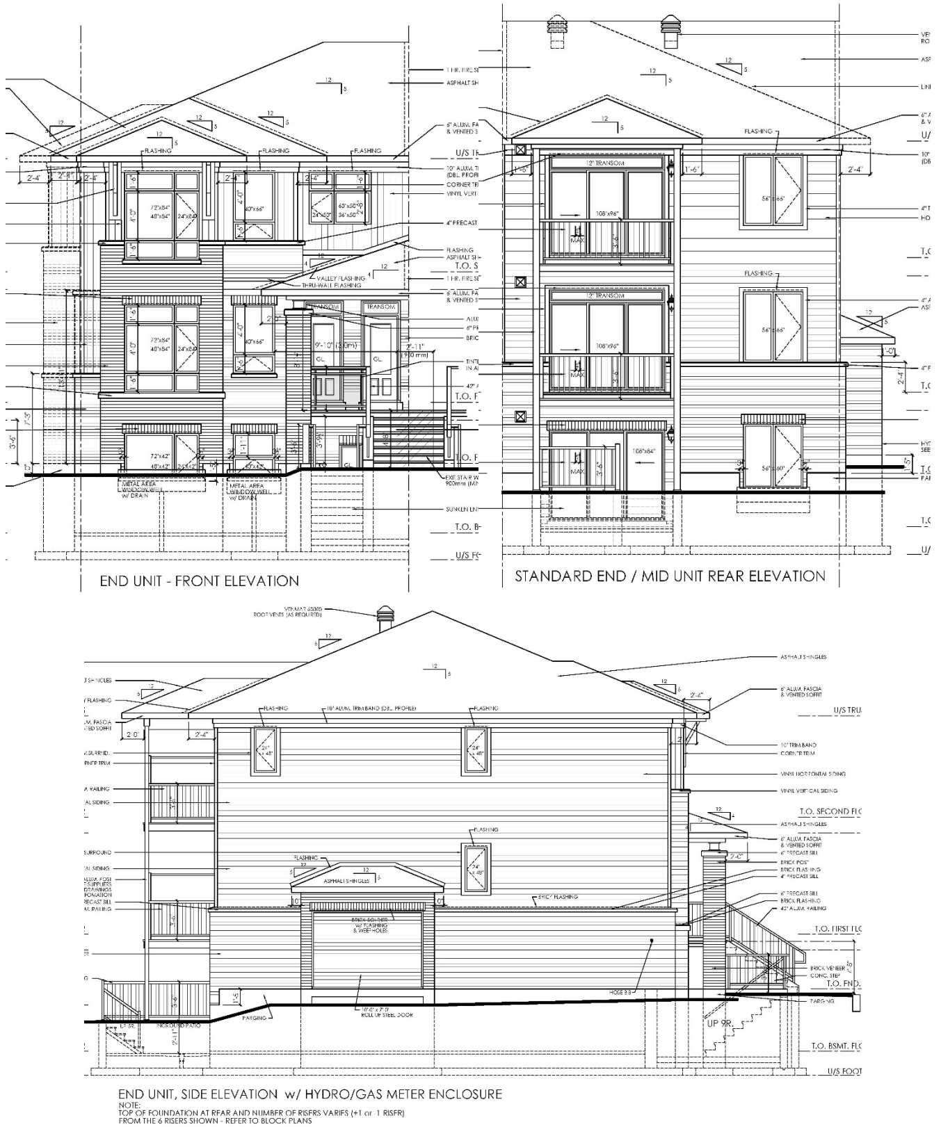
Figure 7. Sample Front (above left), Rear (above right), and Side (below) Stacked Townhouse Elevations (Terrace Flats)
