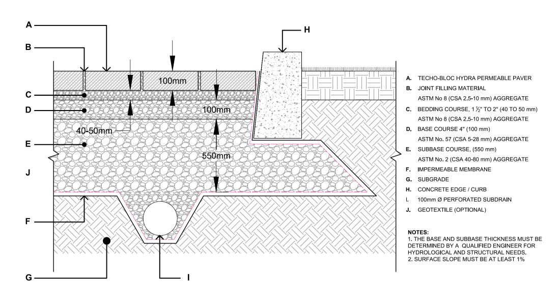
PERMEABLE PAVEMENT DETAIL (NO INFILTRATION)
