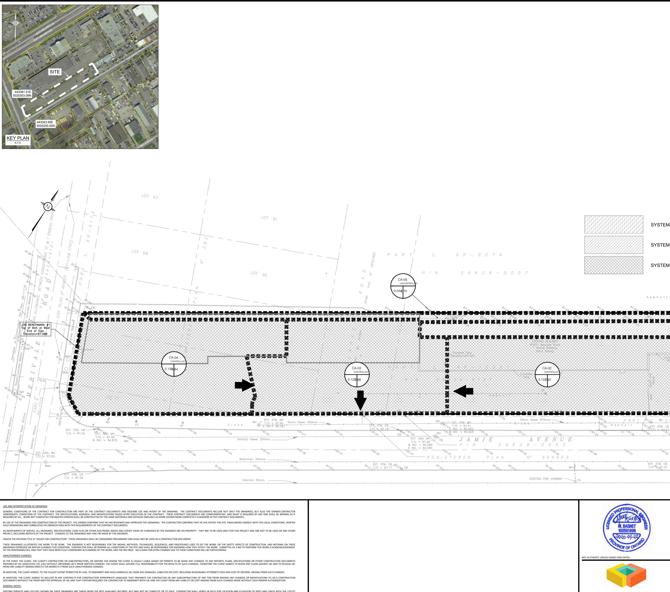
EXISTING SERVICES AND UTILITIES SHOWN ON THESE DRAWINGS ARE TAKEN FROM THE BEST AVAILABLE RECORDS, BUT MAY NOT BE COMPLETE OR TO DATE. CONTRACTOR SHALL VERIFY IN FIELD FOR LOCATION AND ELEVATION OF PIPES AND CHECK WITH THE UTILITY COMPANIES BEFORE DIGGING OR PERFORMING WORK.
