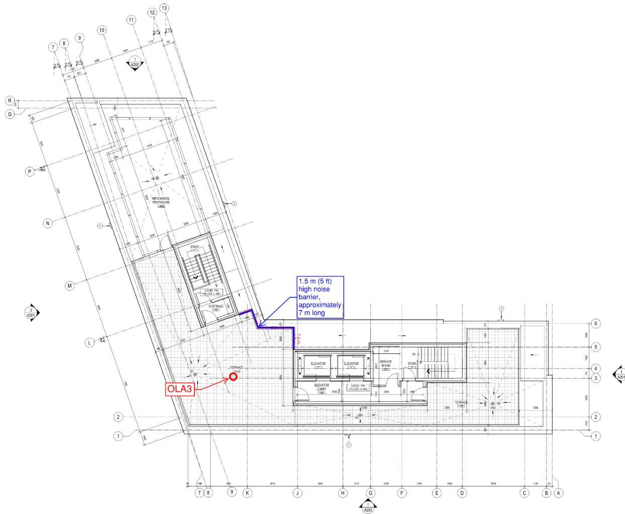
Figure 7: Proposed noise barrier location for OLA3
