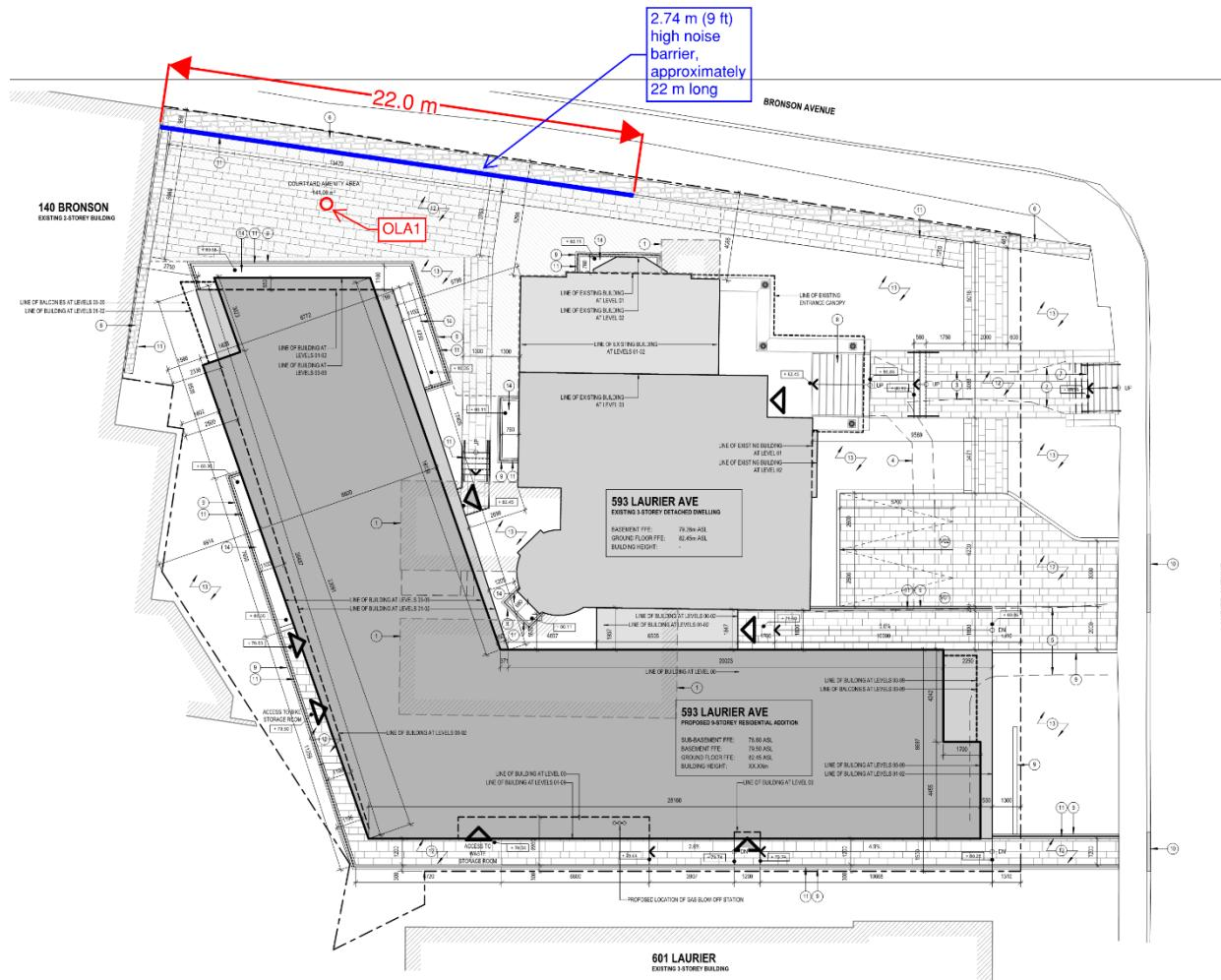
**Figure 6: Proposed noise barrier location for OLA1**
