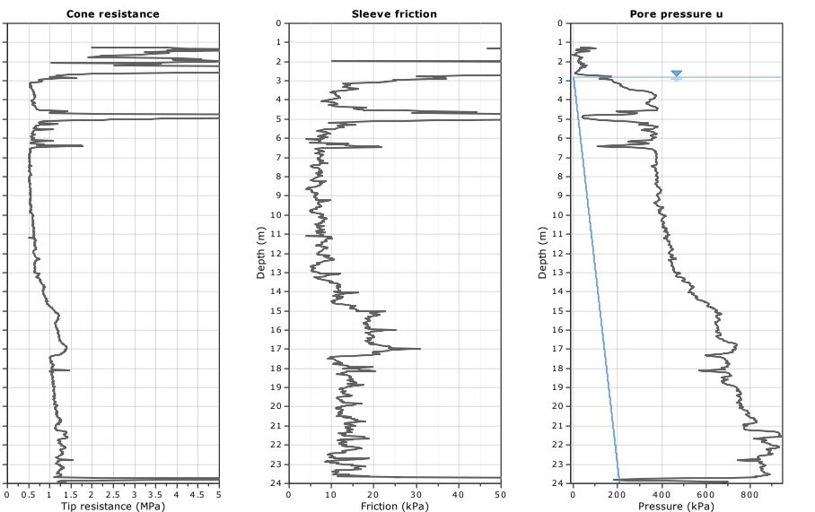
**CPT: 19-10** Total depth: 23.97 m, Date: 19/12/16 Surface Elevation: 77.39 m
