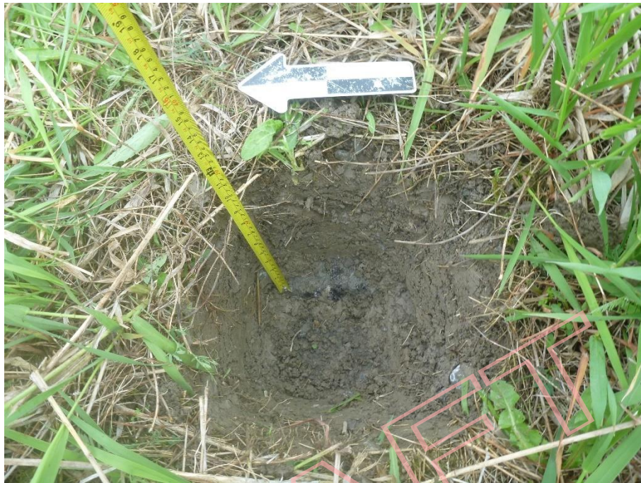
Image 7: Test pit containing approximately 28 cm of mottled grey and orange brown clay fill over layer of very compact grey gravels, view east.
