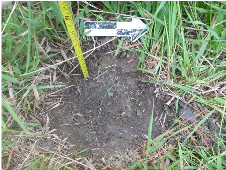
Image 5: Test pit containing approximately 20 cm of mottled orange brown clay fill mixed with gravels, view west. A
