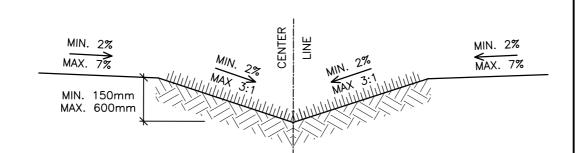
SECTION SWALE AS PER CITY OF OTTAWA DRAWING S29 N.T.S.
