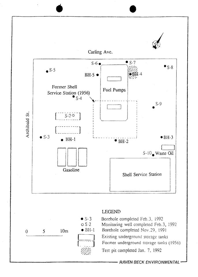
Figure 1 Site Plan of Shell Service Station, 1330 Carling Avenue
