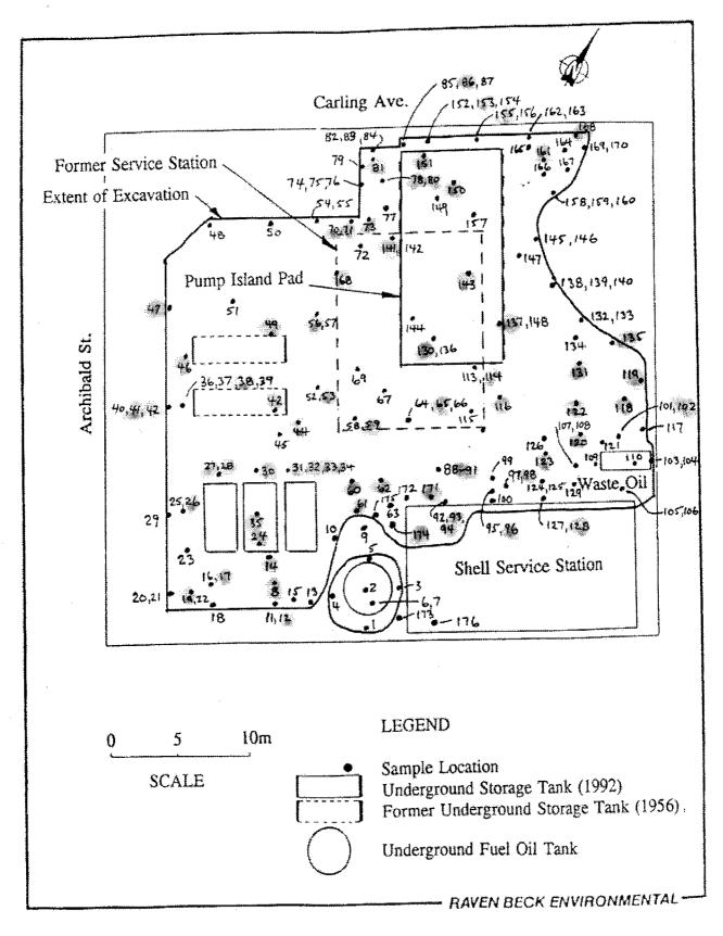
Figure 2 Extent of Excavation and Sampling Locations
