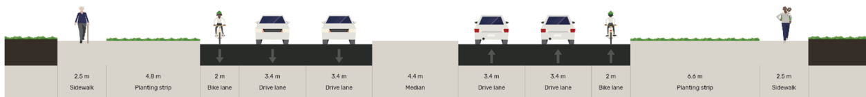
Figure 4-1. Hazeldean Road (west of Fringewood) – Existing Cross-Section
