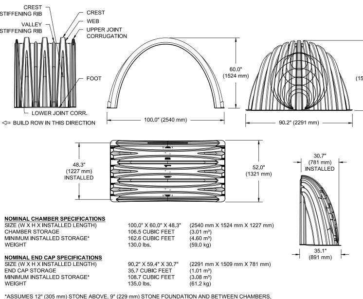
STUBS AT BOTTOM OF END CAP FOR PART NUMBERS ENDING WITH "B" STUBS AT TOP OF END CAP FOR PART NUMBERS ENDING WITH "T" END CAPS WITH A WELDED CROWN PLATE END WITH "C" END CAPS WITH A PREFABRICATED WELDED STUB END WITH "W"
