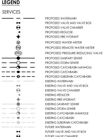
FUTURE VALVE CHAMBER **FUTURE REDUCER** FUTURE FIRE HYDRANT FUTURE SANITARY SEWER FUTURE STORM SEWER \_\_\_\_ FUTURE CATCHBASIN MANHOLE FUTURE CATCHBASIN ----FUTURE SUBDRAIN CATCHBASIN
